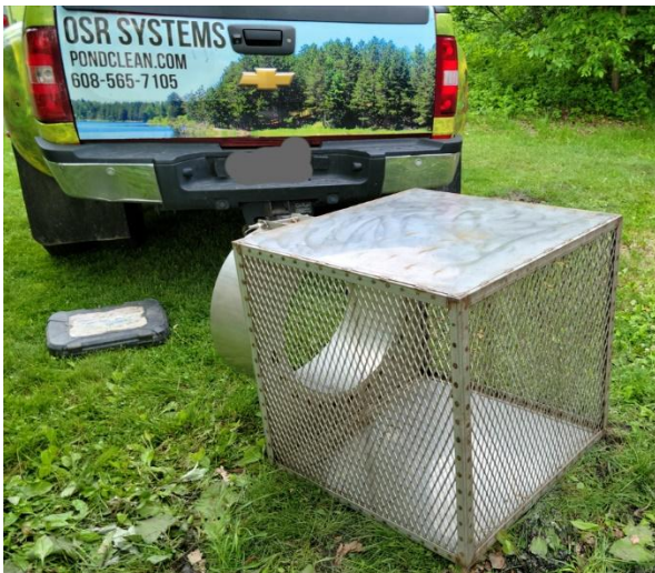
New intake screen awaiting installation
